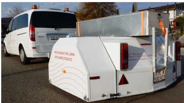
Figure 1: Modified CPX trailer to apply the required weight according to the tyre's load index.
