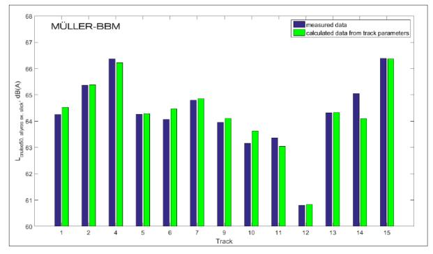
Figure 3-15: Comparison of calculated levels (green bars) according to equation (4) and measured cruise-by sound levels at 50 km/h [Richartz et al., 2019].
