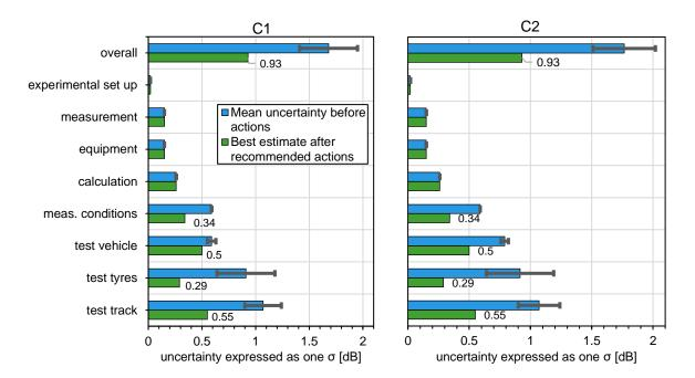
Figure 7-1: Uncertainty contributions per uncertainty group – expressed as standard deviations – for the current tyre noise label procedure (minimum and maximum estimation) and for the situation after implementation of the STEER actions in the procedure; calculation for the C1 tyres (left) and for the C2 tyres (right)
