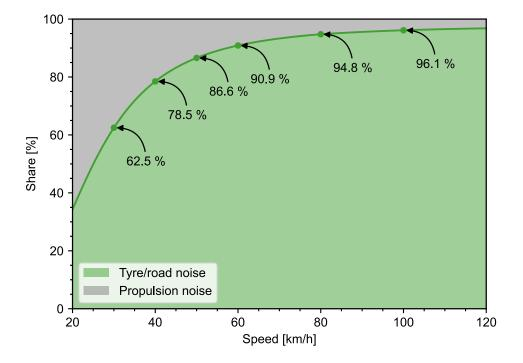
Figure 1-10: Distribution of tyre/road vs propulsion noise. Calculated using Switzerland's road noise calculation model sonROAD18 [Heutschi et al., 2018] for a typical traffic distribution with 8 % heavy vehicles.
