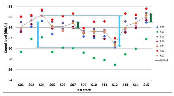
Figure 3-12: Cruise-by levels at 50 km/h, for seven tyres on 13 different ISO test tracks [Richartz et al., 2019]. See the text for further information.
