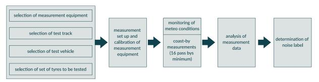
Figure 2-2: Schematic representation of the noise labelling procedure.
