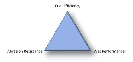
Figure 6-2: The tyre performance "Magic Triangle", consisting of abrasion resistance, wet grip performance and fuel efficiency. Noise is an additional parameter which has to be considered, which may have an impact on the other parameters.
