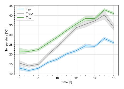
Figure 3-4: Average temperature profiles during a 9-day measurement campaign (with 95 % confidence intervals)
