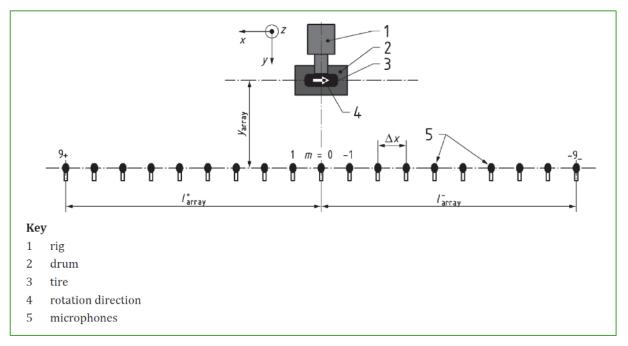
Figure 4-5: Set-up of measurements according to ISO/DIS 20908. The Yarray distance is assumed to be at least 1.75 m.
