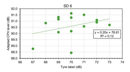
Figure 4-13: Adapted CPX levels on 6 mm surface dressing (SD 6) as a function of the tyre (noise) label [Hammer et al., 2018]
