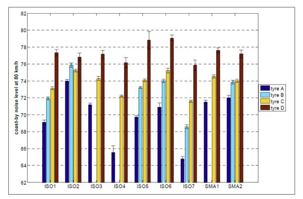
Figure 3-10: Coast-by levels at 80 km/h for all tyres at each test track; error bars show 95 % confidence intervals.
