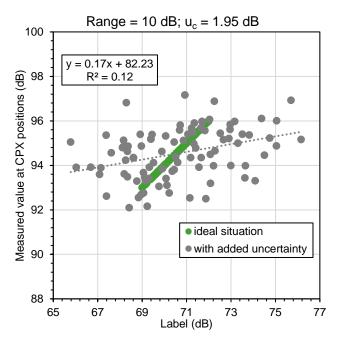
Figure 2-4: Illustration of the effect of adding uncertainties to true values using Monte Carlo simulation of correlation between a tyre label with the calculated uncertainties added to coast-by measurements (actual range of true label = 3 dB and uncertainty of label = 1.95 dB, uncertainty on CPX measurement = 0.58 dB, all expressed as standard deviations).
