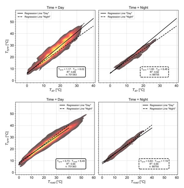
Figure 3-5: Relationships between *T*<sub>tyre</sub> and *T*<sub>air</sub> (upper part), and *T*<sub>road</sub> (lower part) during daytime with varying amount of solar radiation (left) and during night-time, i.e., without solar radiation (right).
