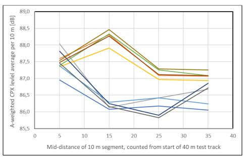
Figure 3-17: A-weighted CPX levels as a function of distance from start of drive lane (average per 10 m distance). The upper five curves are for the eastern wheel track and the five lower curves are for the western wheel track. The measurements were made on a two-month-old ISO test track laid 2020 near Skövde in Sweden.
