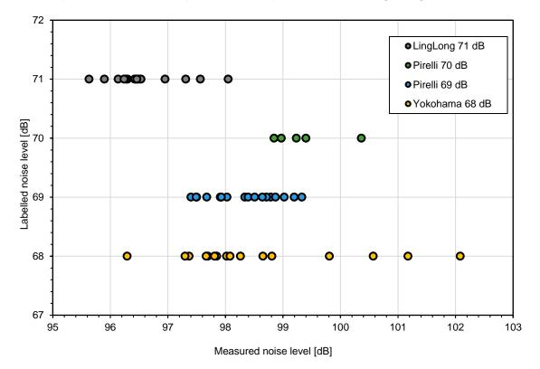
Figure 4-4: Distribution of measured noise levels for each of the tyre selections (with each tyre's label level on the ordinate). One symbol for each tyre. The two Pirelli selections are for the same tyre line but separated for the labels 69 and 70 dB.
