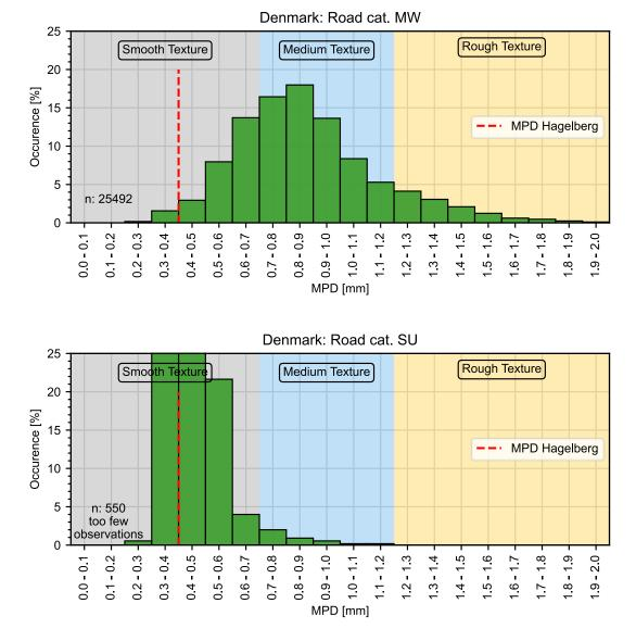
Figure 4-7: Distribution of MPD values in Denmark on highways (top) and on local roads (bottom). Red line is the MPD value of the Swedish ISO test track.
