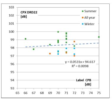
Figure 4-11: Measured CPX levels on SMA 11 road surface as a function of tyre label values issued by the tyre manufacturer. Figure copied from [Kragh et al., 2015].
