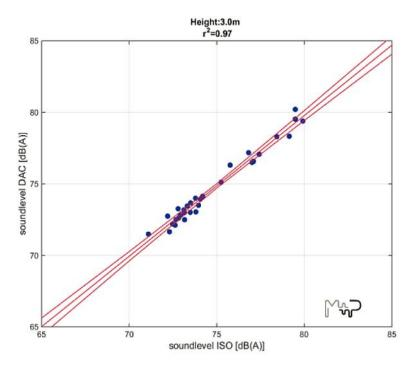
Figure 4-12: Measured coast by noise levels of truck tyres on the ISO test track versus noise levels measured on DAC 16 [Blokland et al., 2015].
