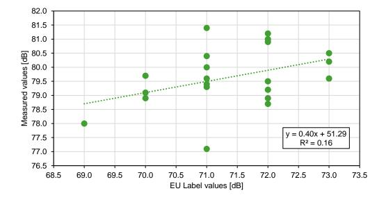
Figure 4-10: Regression analysis of "EU label" values and measured noise levels on the SMA 11 road surface. Graphics by the authors with data from [Berge, 2005].
