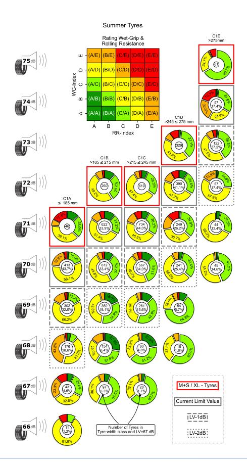
Figure 6-4: Rating of C1 **summer tyres** (Switzerland 2021), sorted according to their tyre width (hypothetical X axis, rated A-E according to EC 661/2009). On the hypothetical Y axis, the noise limits are depicted. The colours indicate the related Wet grip / Rolling resistance Index as defined by the matrix.<sup>17</sup>.
