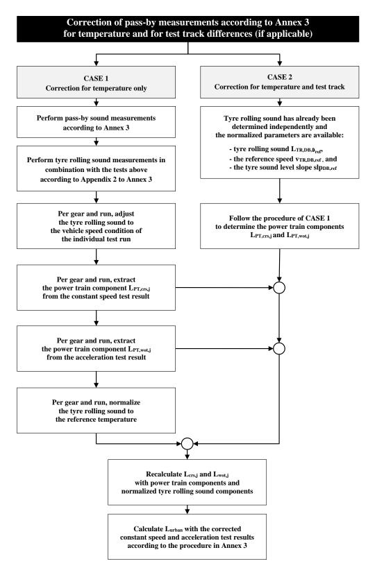
Figure 2-1: Flowchart for vehicles tested according to R51.03, Annex 3 – Correction of pass-by measurements for temperature and test track, if applicable. Flowchart from [GRBP, 2021a]
