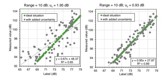
Figure 7-2: Demonstration of the effect of the reduced uncertainty before (left graph) after implementing (right graph) the STEER proposals by Monte Carlo simulation of the relation between the noise label and CPX measurements.
