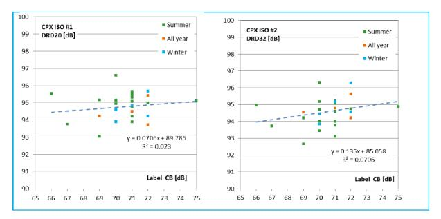
Figure 2-5: Measured CPX levels on two ISO test tracks as a function of the tyre label values issued by tyre manufacturers [Kragh et al., 2015].
