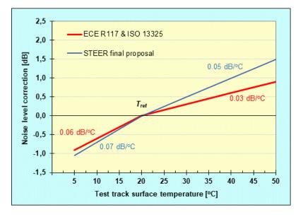
Figure 3-8: Illustration of an alternative temperature correction model for measurements of tyre category C1, in accordance with R117 and ISO 13325. In this case the road surface is the reference surface specified in ISO 10844.
