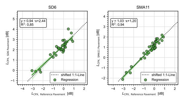
Figure 4-14: Regression analysis between tyre CPX levels measured on the reference surface vs. the test surfaces. (Left: SD6, Right SMA 11). (Normalized values)
