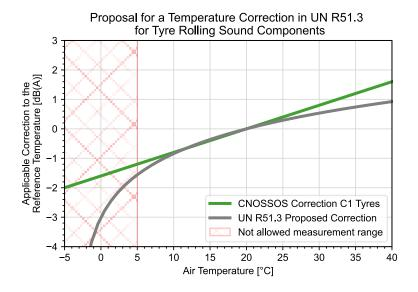
Figure 3-6: Proposed temperature correction for R51.03, compared with the present correction for C1 tyres in CNOSSOS-EU. The figure is from [OICA, 2021] but has been edited by the authors without changing any data.
