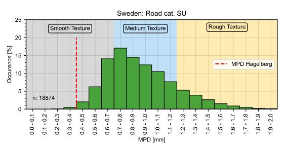
Figure 4-8: Distribution of MPD values in Sweden on highways (top) and on local roads (bottom). Red line is the MPD value of the ISO test track.
