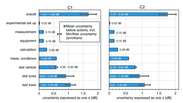
Figure 2-3: Uncertainty contributions per uncertainty group for the C1 (left) and C2 tyres (right) when labelled under the current tyre noise labelling procedure. Note that σ stands for standard deviation.
