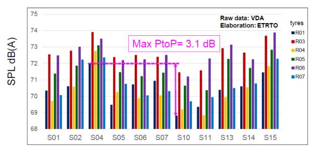
Figure 3-14: The VDA RRT results elaborated by ETRTO showing track-to-track variations at 80 km/h [ETRTO, 2019].
