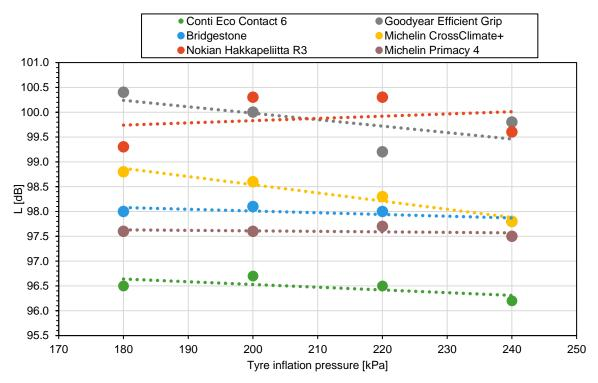
Figure 4-1: Tyre inflation pressure influence on measured noise levels for six C1 tyres.
