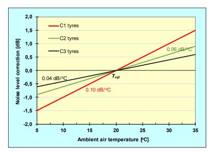
Figure 3-7: Illustration of the temperature correction model. In this case the data for dense asphaltic surfaces are used for the three tyre categories C1, C2 and C3. Coefficients for other road surface types are listed in Table 3-3.
