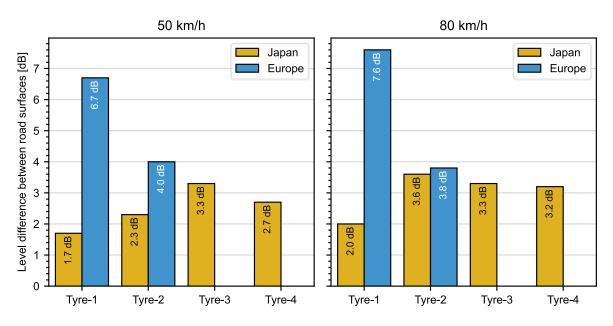
Figure 3-11: Spread of coast-by tyre/road noise levels at 50 km/h (left) and at 80 km/h (right) between the test tracks for the four tyres in Japan in yellow and the European tyres B and C in blue. Graphics by the authors, data from [JSAE, 2006].
