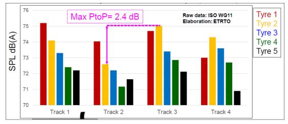
Figure 3-13: Results of the RRT by ISO/TC 31/WG 11, elaborated by ETRTO. Results show track-to-track sound level variation at 80 km/h [ETRTO, 2019].
