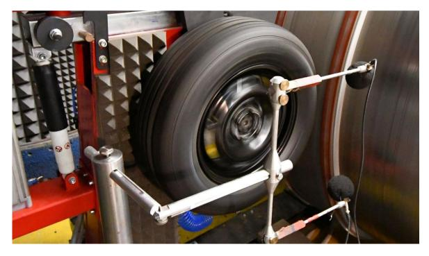
Figure 4-2: The laboratory drum facility at the GUT in Gdansk. The drum diameter is 2.0 m. An overview above and a zoom-in on the tyre/drum contact area below. Note the position of the microphones.
