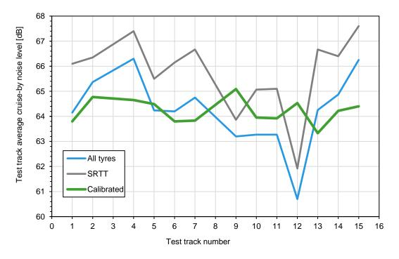
Figure 3-16: Comparison of measured cruise-by sound levels at 50 km/h for each test track (average for all tyres excl. the slick tyre in red) and the corresponding sound level for each test track after implementing the Reference Tyre
